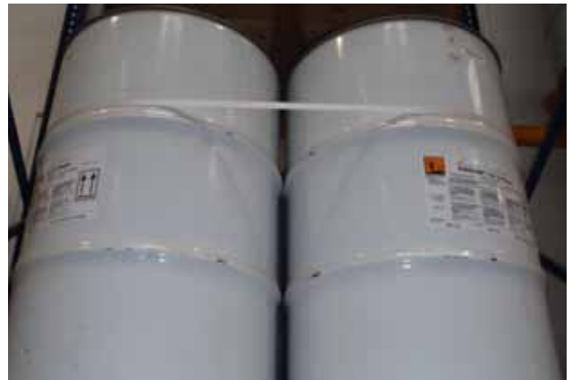
Photo 6-18 - Drums holding 240 kg of HCFC-141b intended for use as foam blowing agent
