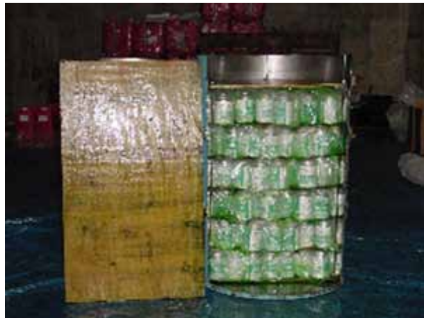
Photo 5-11d Aspect of concealment re-created after cutting the oil drum vertically.
