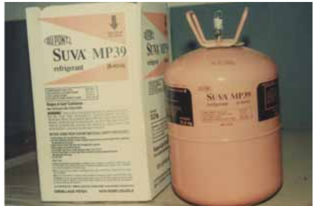
Photo 6-2 - Disposable cylinder with SUVA MP39 - an R-401 refrigerant blend containing HCFCs.
