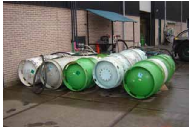
Photo 6-20 - One tonne (1000 kg) capacity pressurised cylinders
