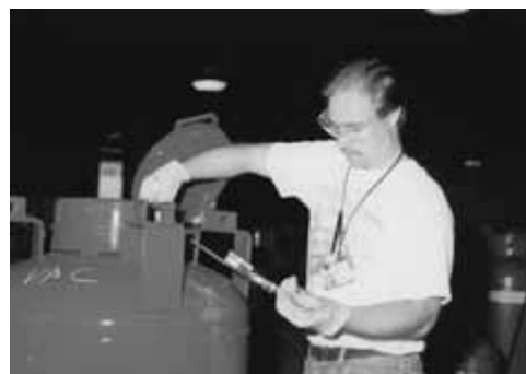
Photo 7-2. Conducting a temperature-pressure test.
