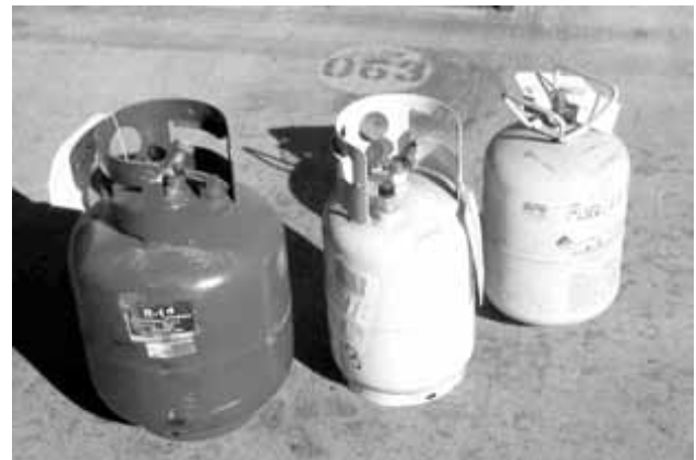
Photo 6-12 - 50 (22.7kg) and 30 lb (13.6kg) reusable cylinders; 30 lb (13.6kg) disposable cylinder.
