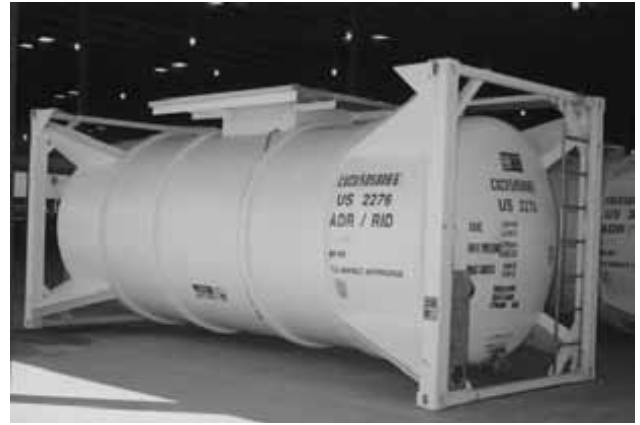
Photo 6-16 - ISO tanks allow for multimodal transport of large quantities of refrigerants.
