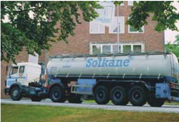
Photo 6-19 - Truck cistern used for transportation of large bulk quantities of HCFC-141b
