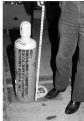
Photo 6-10 - "Recovered" R-502 (mixture of 49 per cent HCFC-22 and 51 per cent CFC-115) cylinder.
