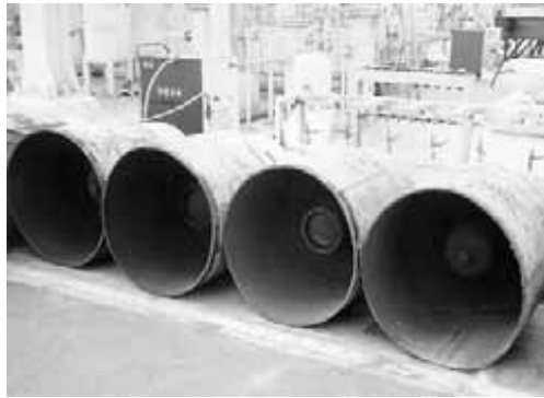
Photo 5-2 . View of the small HFC-134a cylinders after removing the CFC-12 refrigerant and cutting open the main containers.
