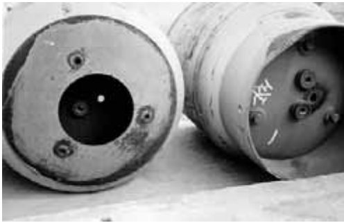
Photo 5-1. The access points to the main CFC-12 container become visible only after the double-layered container is cut open.
