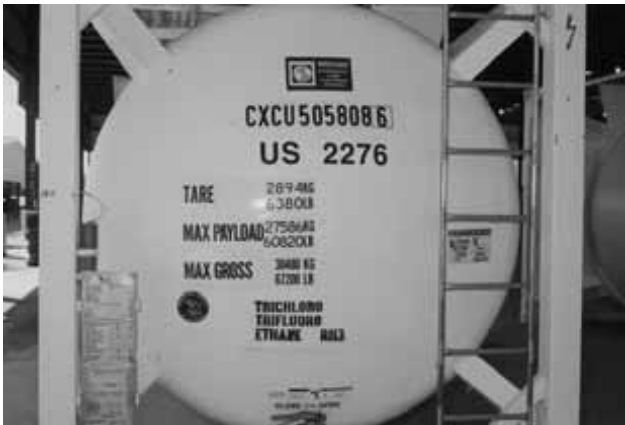
Photo 6-17 - Front end of an ISO tank (see box for example of ISO tank labelling).
