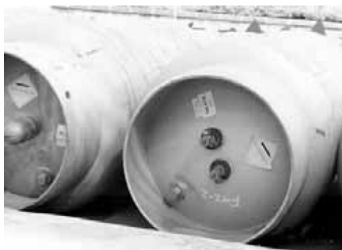
Photo 5-4. View of the seized CFC-12 containers declared and labelled as HFC-134a.
