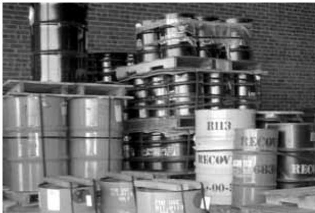
Photo 6-11 - Various low-pressure containers.
