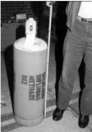
Photo 6-9 - Example of CFC-12 cylinder, dichlorodifluoromethane.
