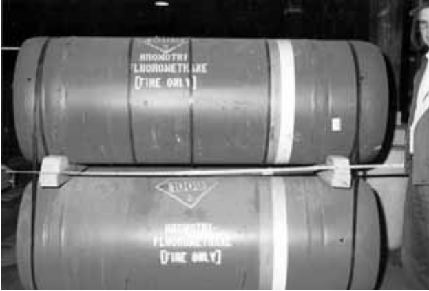
Photo 6-21 - Barrel of halon 1301 (bromotrifluoromethane).
